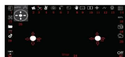
1. Exit 2. Gravity Mode 3. Roll 4. Gesture Control (Take picture ; Video ; ) 5. Switch camera 6. Follow Mode 7. Picture in Picture 8. Palm Control Flight 9. Panorama 10. Split Screen 11. Headless Mode 12. Flip 13. Flip Preview 14. Menu 15. Calibration 16. Speed 17. Album 18. Take Photo 19. Entertainment 20. Video 21. Left Remote 22. Right Remote 23. Take-off and Landing 24. Emergency Stop 25. Show controls 26. Virtual head control
